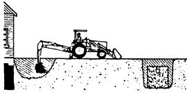
Position the unit so the backhoe swing post is over the centerline of the trench connection. Dig with the backhoe at extreme swing positions, and in as close to the stabilizers as possible. Pile the spoil on the opposite side of the trenches.
